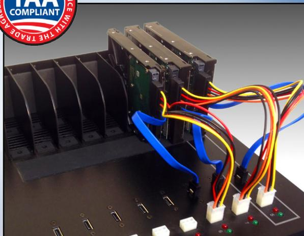
*This TAA Compliant Hard Drive Duplicator is easy to use, and can clone up to 15 hard drives or solid state drives simultaneously. As a stand-alone unit without the need to connect to a computer, the KanguruClone 15HD SATA Pro Drive Duplicator is perfect for large duplication jobs.*
